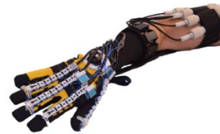
Figure (2-6) The SPAR Glove combines a novel glove-based exoskeleton with intent detection at the wrist [14].
