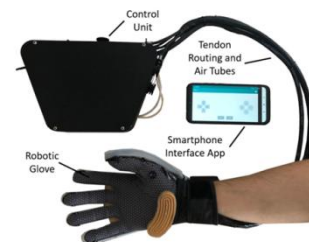
Figure (2-7) The hybrid exoskeleton glove is equipped with a tendon-driven system for finger flexion, pneumatic actuators for finger abduction, and an inflatable, telescopic extra thumb for grasp quality enhancement.
