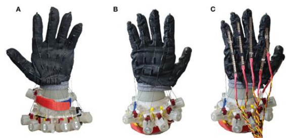
Figure (2-4) Anthropomorphic robotic hand with glove for external muscles and attached motors. (A) The front view of the robotic hand. (B) The rear view of the robotic hand. (C) A robotic hand equipped with flexible sensors for posture estimation. [19]
