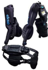
Figure (2-20) The EVO (Ekso Bionics Holdings Inc, California, USA) upper limb exoskeleton is used as a wearable device with three levels of passive assistance [40].
