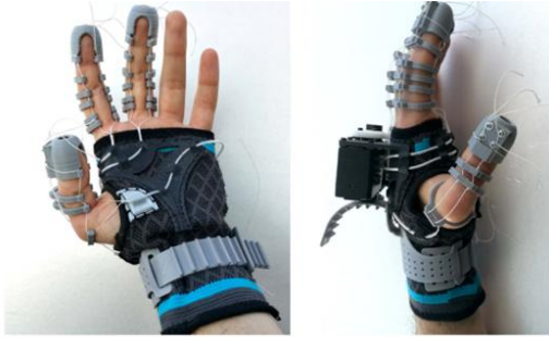
Figure (2-8) Preliminary prototype of the compact soft exoskeleton. Actuator and tendon transmission are arranged around the palm and hand dorsum, with no remote Mechanical parts [24].
