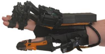
Figure (2-5) HandMATE device. Individually actuated fingers and thumb shown. Electronics box is affixed to back of splint [20].
