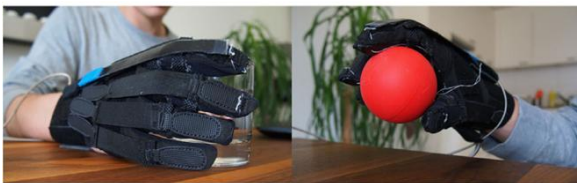
Figure (2-12) The soft, synergy-based robotic glove for grasping assistance [31] .
