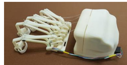
Figure (2-11) The figure shows the two blocks of the HES modular structure: on the left, the fingers' mechanisms module, and on the right, the motor and control one [26].
